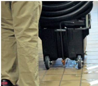
Dispense fresh solution through throttle spigot on the rear of the Trolley-Bucket.
